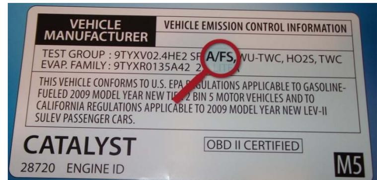
\* Note: Air/Fuel sensors are before the catalytic converter
